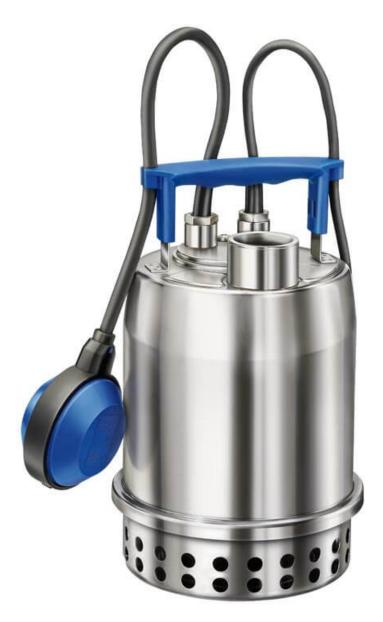
The stainless steel submersible pumps from the TOP 71 range are especially suitable for handling clean, clouded or slightly contaminated water, for example swimming pool water, ground water, rainwater and clarified sludge. All wetted parts are made from stainless steel 1.4301. The non-return valve is included in delivery.
