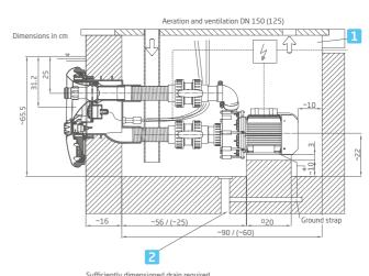
Sufficiently dimensioned drain required. Dimensions in brackets [ ] only for BADU 21-81/33 1 $^{\sim}$  and BADU 21-81/34 3 $^{\sim}$
