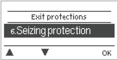
The menu "6. Protections/Protective functions" can be used to activate and set various protective functions.
