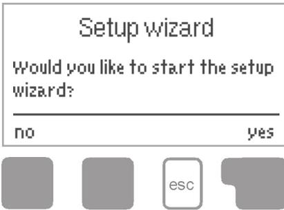
The first time the controller is turned on and after the language and time are set, a query appears as to whether you want to parameterise the controller using the commissioning help or not. The commissioning help can also be terminated or called up again at any time in the special functions menu. The commissioning help guides you through the necessary basic settings in the correct order, and provides brief descriptions of each parameter in the
