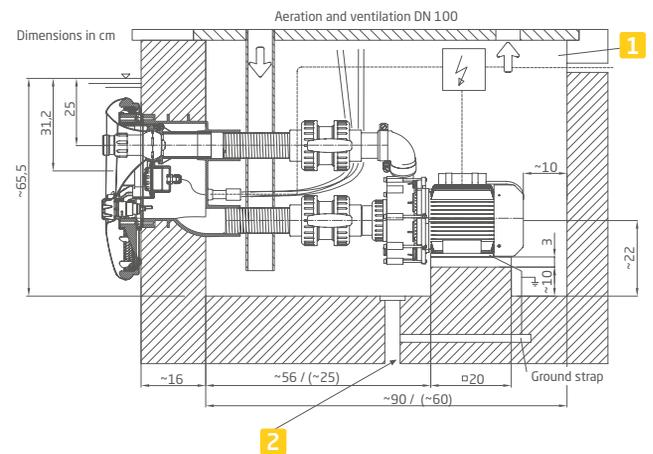
Sufficiently dimensioned drain required
