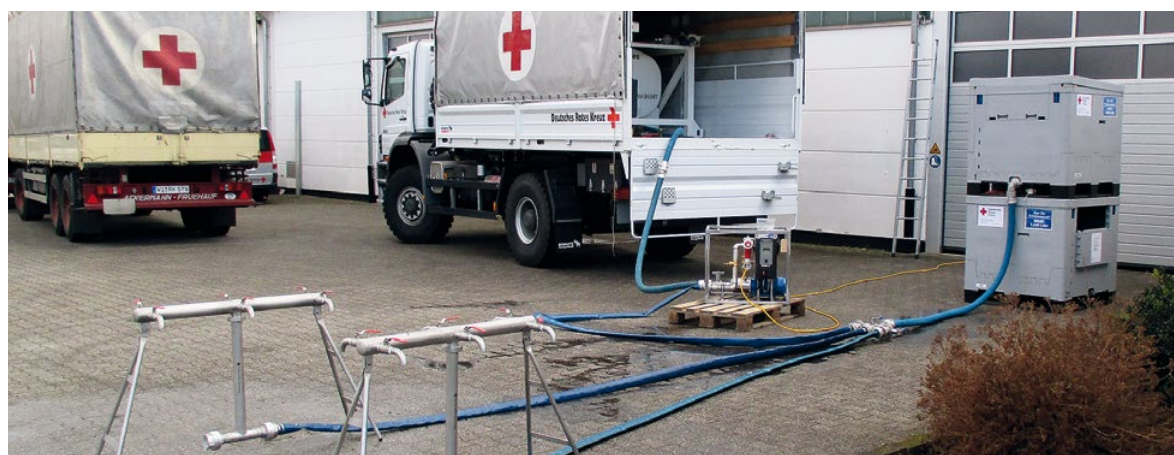
The German Red Cross's test construction for mobile drinking water supply with the SPECK Minicell. Photos: SPECK Pumpen
